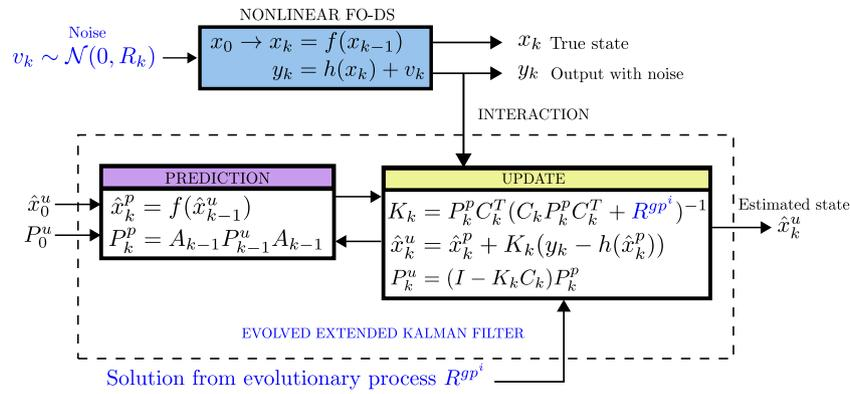
**Fig. 3.** Layout of the EEKF. The construction of the EEKFs is based on the analytic behaviors framework, that solves the estimation task in the presence of uncertainty introduced by the noise  $v_k$ . The solutions  $R^{gp^i}$ ,  $i = 1, \dots, m$  are optimized analytic functions derived from an evolutionary process applied to the filter.
