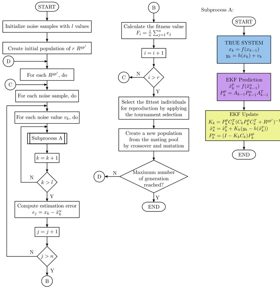
**Fig. 4.** Evolutionary process for the synthesis of optimized analytic functions  $R^{gp^i}$ ,  $i = 1, \dots, m$  as estimations of the unknown covariance value  $R_k$  for the additive noise  $v_k$ . The analytic functions are applied into the structure of EKF aiming to solve the estimation task of a nonlinear FO-DS.
