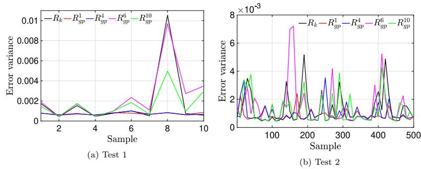
**Fig. 7.** Error variance for each noise sample in Test 1 7(a) and Test 2 7(b). In Fig. 7(a) note that the highest fluctuation in sample 8 is due to the natural response of the filter to that particular noise sample. Despite this, the performance produced by the conventional EKF is not as good as the one provided by our proposal.
