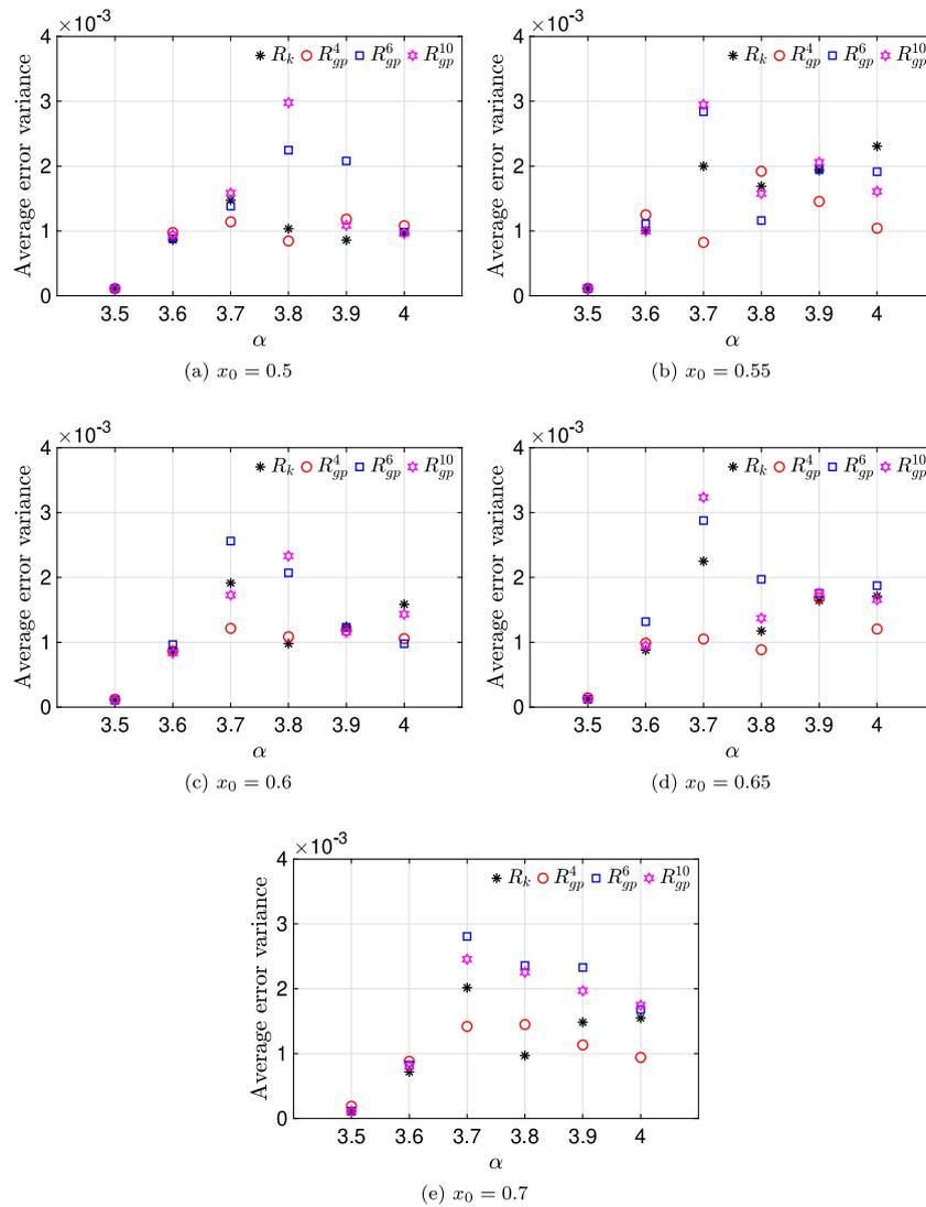
**Fig. 8.** Robustness analysis of the discovered solutions against the conventional EKF. Each solution is tested with five different initial conditions and for six different values of parameter  $\alpha$ . The average error variance is shown in each case.
