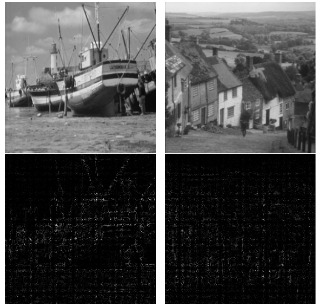
Figure 6: At the top, the images corrected using the Von Neumann neighborhood. At the bottom, the difference, increased ten times, between the reconstructed and the original image.
