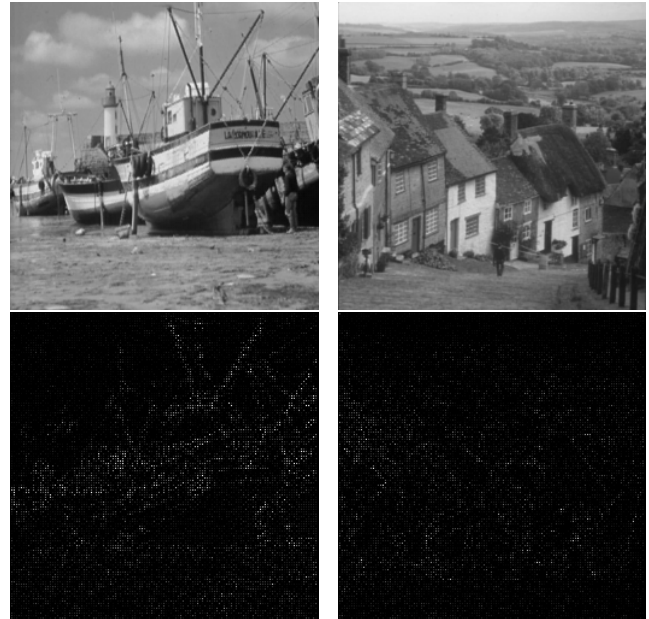
Figure 5: At the top, the images corrected using the Moore neighborhood. At the bottom, the difference, increased ten times, between the reconstructed and the original image.
