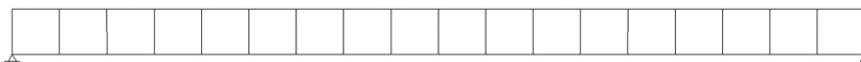
Fig. 5. Sample truss design evolved using DO-GE. Experimental variables are: span: 24 m, style = Vierendeel, height = span/19, r = 9 .
