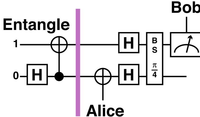
Figure 8.14. A gate array diagram for an evolved protocol for communicating one classical bit through a  $BS(\frac{\pi}{4})$  gate in the context of prior entanglement. The entanglement-generating gates, to the left of the vertical bar, were included in the embryo to which the developmental process was applied.
