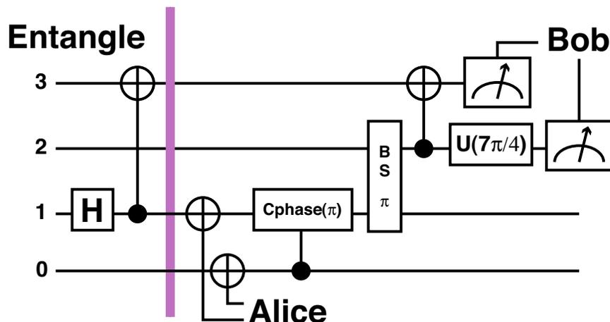
Figure 8.15. A gate array diagram for an evolved protocol for communicating two classical bits through one application of a  $BS(\pi)$  gate in the context of prior entanglement. This is a form of quantum superdense coding re-discovered by genetic programming. The entanglement-generating gates, to the left of the vertical bar, were included in the embryo to which the developmental process was applied.
