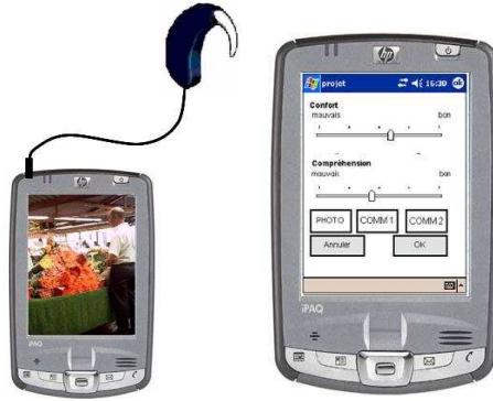
Fig. 9. A sampling software has been developed on a PDA that the patient plugs directly onto the CI processor in order to sample the exact sound that is received by the processor.
