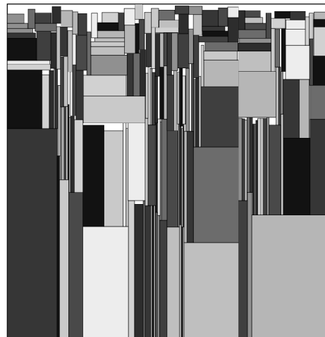
Fig. 17. Packing obtained by the best evolved heuristic on instance PathP4, to a height of 104.1. similar to figure 16, post-processing would improve this solution further, by laying the tallest piece on its side
